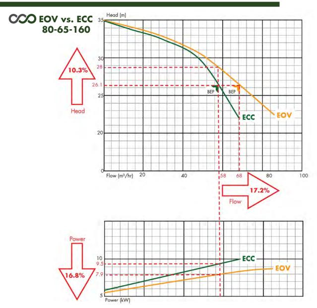
The New EOV range is based on a radically redesigned volute casing and impeller featuring an improved vane design that improve efficiencies by up to 35%. Not only are flow rates and discharge pressures increased, these improvements are achieved absorbing considerably less power and reducing your running costs.
