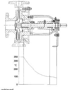
Heat transfer installations have achieved a high level of technical development. Consequently the requirements on pumps handling heat transfer oils have increased regarding operating safety, environmental protection, maintenance and operating costs. The Sterling SIHI ZTN pump, based on many years of experience and on the latest technical know-how, fully complies with these requirements.
