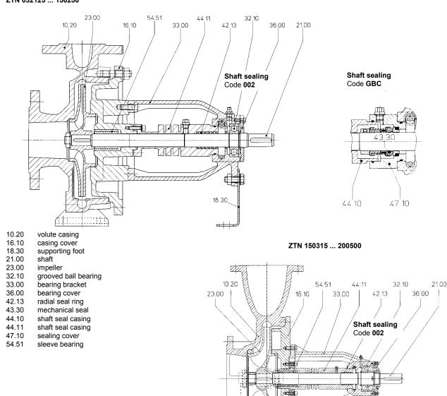
Heat barrier / shaft sealing / bearing
